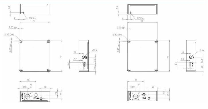
Connector: Positive center plug OD: 3.5mm, ID: 1.3mm, L: 9mm
